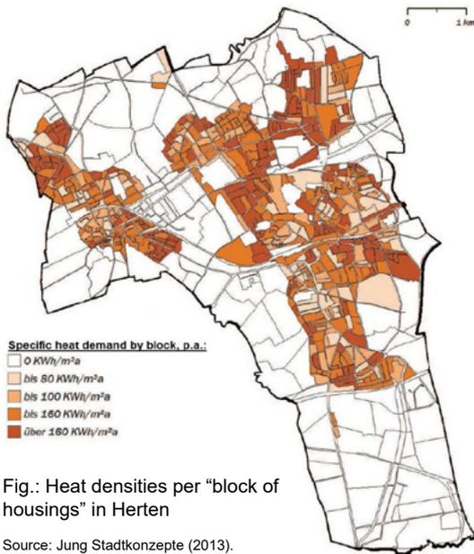
Fig.: Heat densities per “block of housings” in Herten
